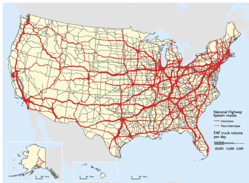
FIGURE 12 Average Daily Long-Haul Truck traffic on the National Highway System: 2011
